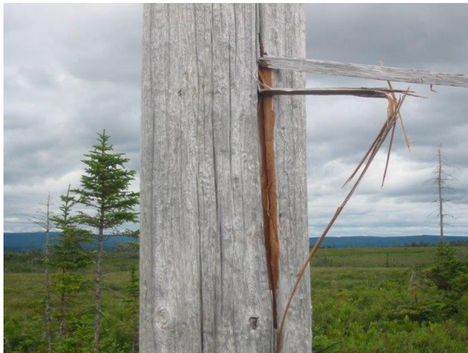
Figure 14 – Pole Shell Separation Showing Exposed Inner Wood
