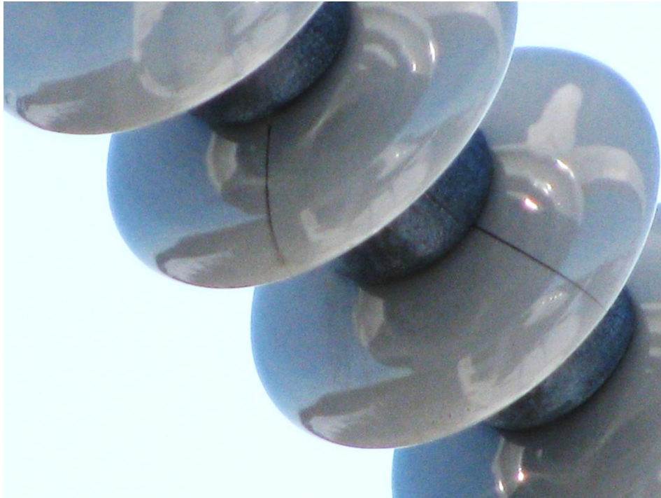
Figure 33 – Cracks in COB Type Insulator
