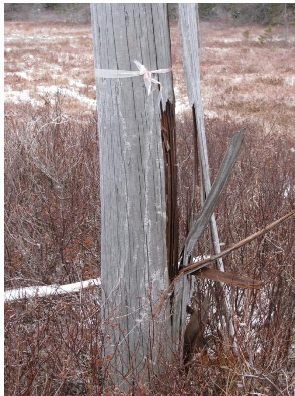
Figure 40 – Outer Shell Layer Separation
