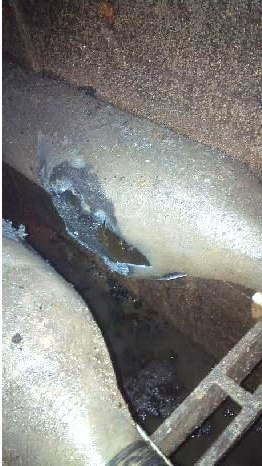
Figure 1 – SLA-09 Faulted Underground Cable
