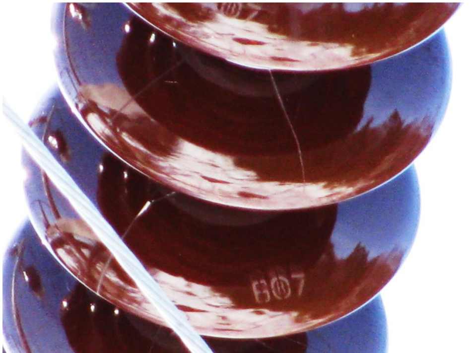
Figure 34 – Cracks in OB Type Insulator
