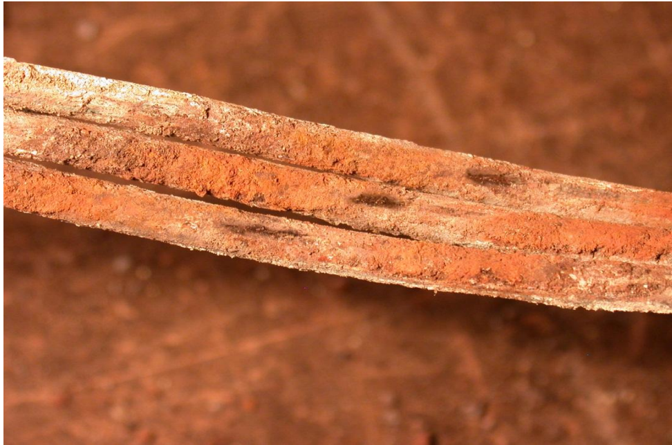
Figure 13: Arc damage on the copper armor wires close to the fault of the failed cable.
