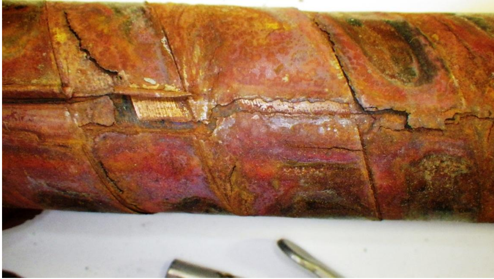
Figure 14: Cracks and corrosion damage on the copper tape of Sample #1 of the failed cable.
