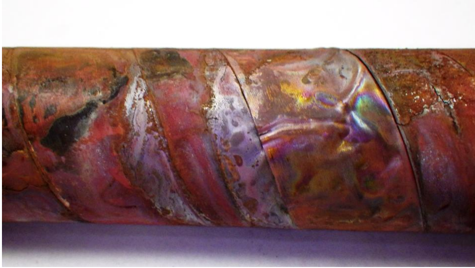
Figure 16: Cracks on the wrinkled area of the copper tape of Sample #1 of the failed cable.
