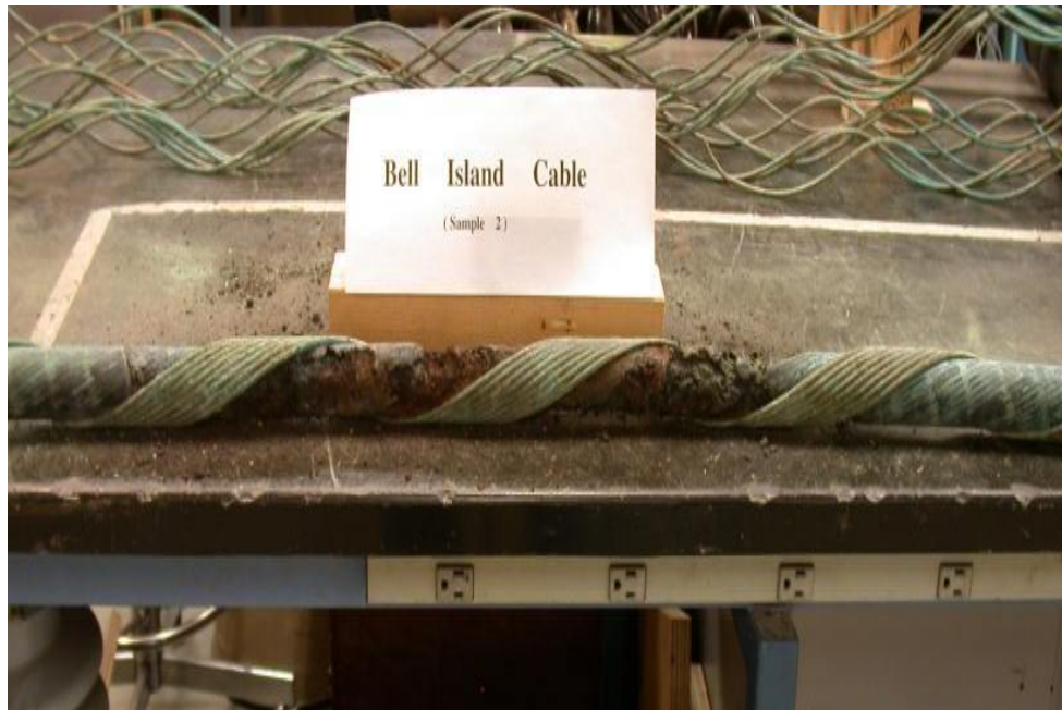
Figure 11: Condition of the failed cable after the partial removal of armor wires.
