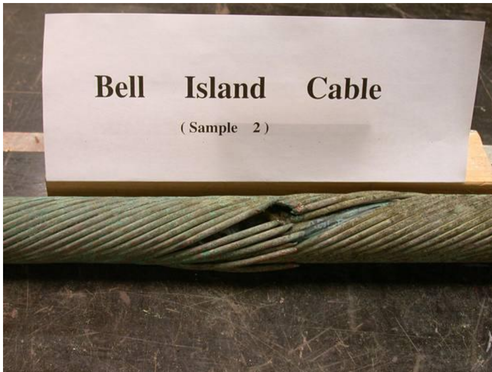
Figure 9: Faulted section of the failed submarine cable.
