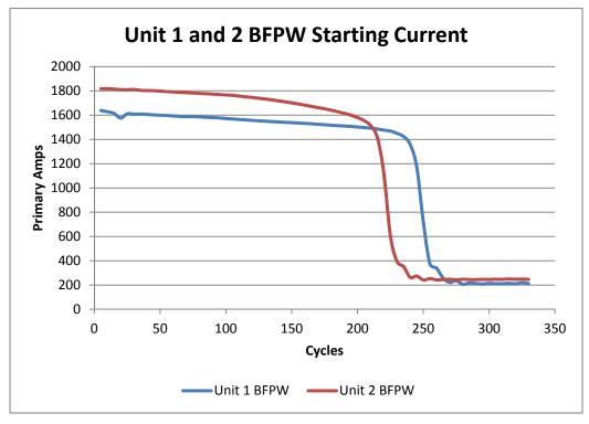
Figure 1 Actual Motor Starting Currents for Units 1 and 2 BFPW
