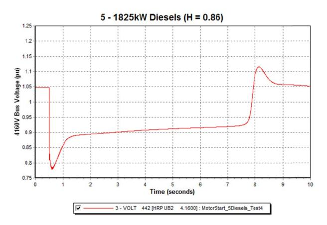
Figure 2 (Motor Starting – 4.16kV Bus Voltage)
