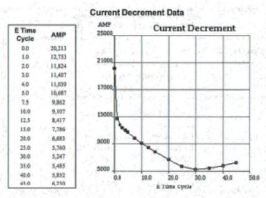
Instantaneous 3 Phase Fault Current: 20213 Amps Instantaneous Line - Line Fault Current: 17909 Amps Instantaneous Line - Neutral Fault Current: 30076 Amps
