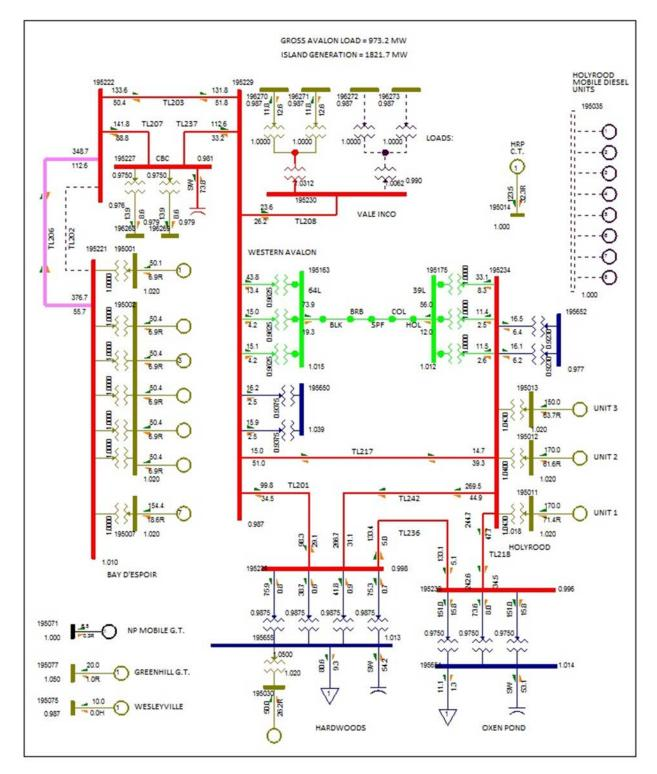
Figure 2 – Avalon Peninsula Load Flow Plot – 2016-17 P90 Peak Load Case Holyrood Diesel Generation Not In Service
