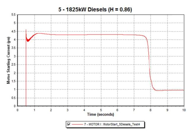
Figure 3 - Motor Starting Current
