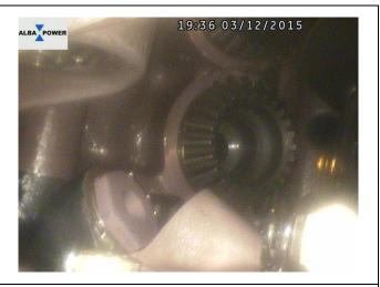
Drive gears Intermediate Case
