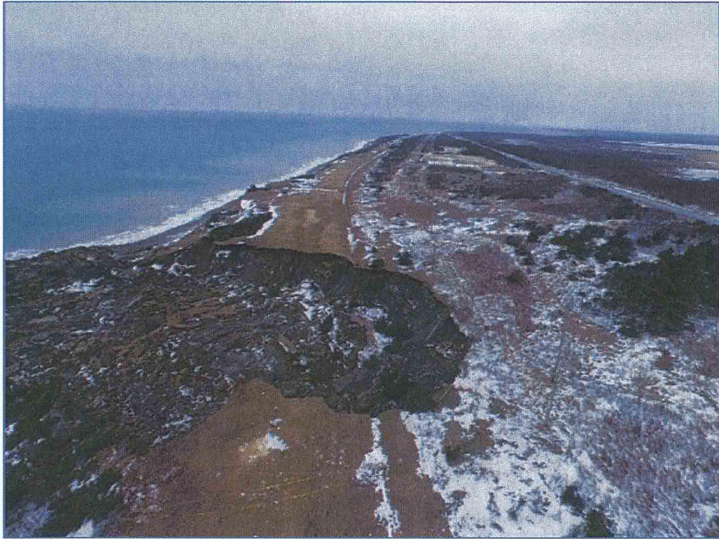
Figure 2: Aerial View of Coastal Landslide near TL 259, TL 227 and Sally's Cove L1
