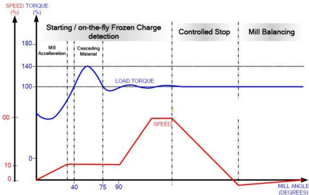
Figure 6: Speed / Torque vs Mill Angle
