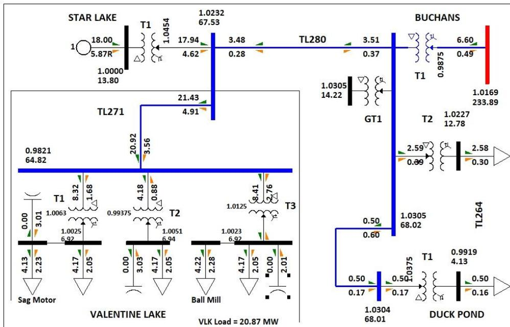
Figure 3: Normal System Operation – 20.87 MW Loading to Meet Voltage Criteria
