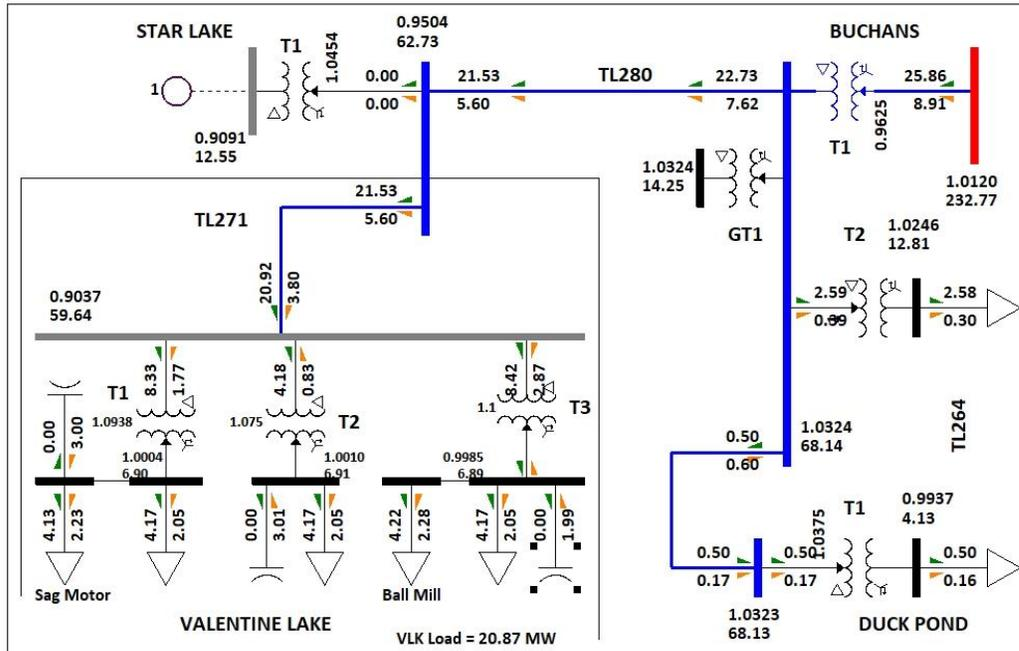
**Figure 4: N-1 Star Lake Generator Out of Service – 20.87 MW Loading to Meet Voltage Criteria**
