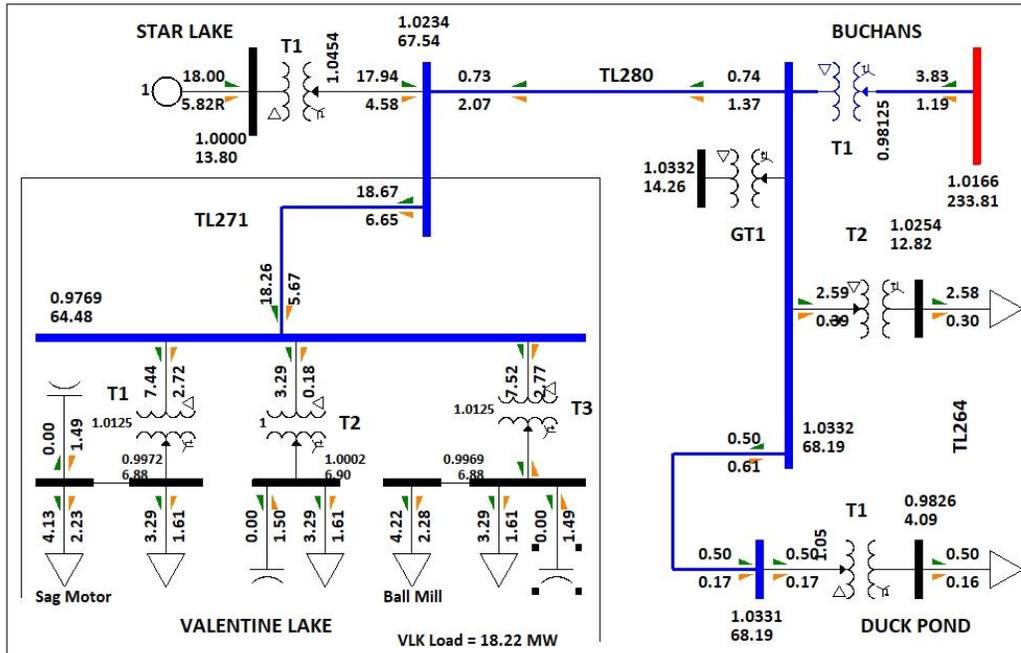
Figure 1: Normal System Operation – 18.22 MW Loading to Meet Voltage Criteria
