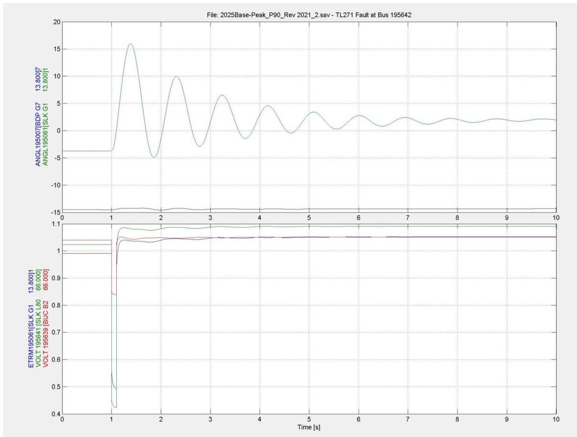
**Figure 14: Dynamic Results of 3 Phase Fault at VTN66 and Trip of TL271 after 6 Cycles**
