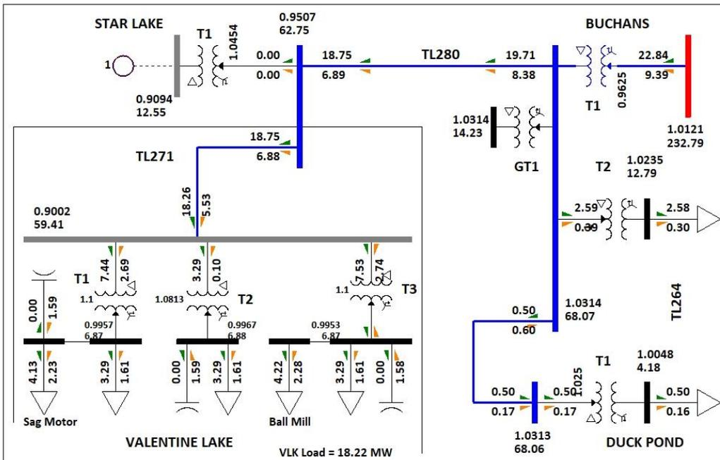
Figure 2: N-1 Star Lake Generator Out of Service – 18.22 MW Loading to Meet Voltage Criteria
