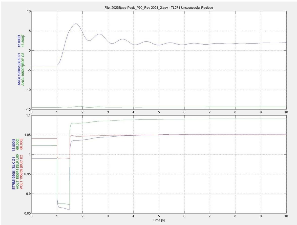
**Figure 15: Dynamic Results of SLG Phase Fault on TL271 near VTN and Trip after 30 Cycles**
