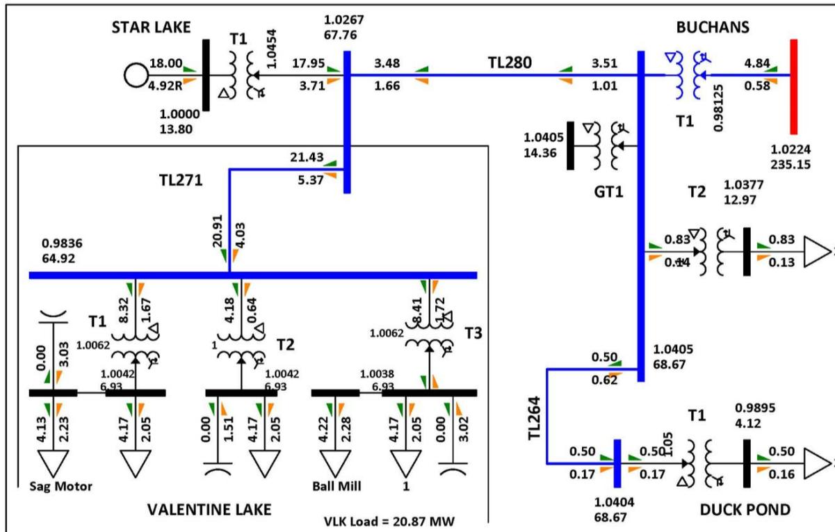
Figure 10: 2024 Light Load Case – Normal System Operation
