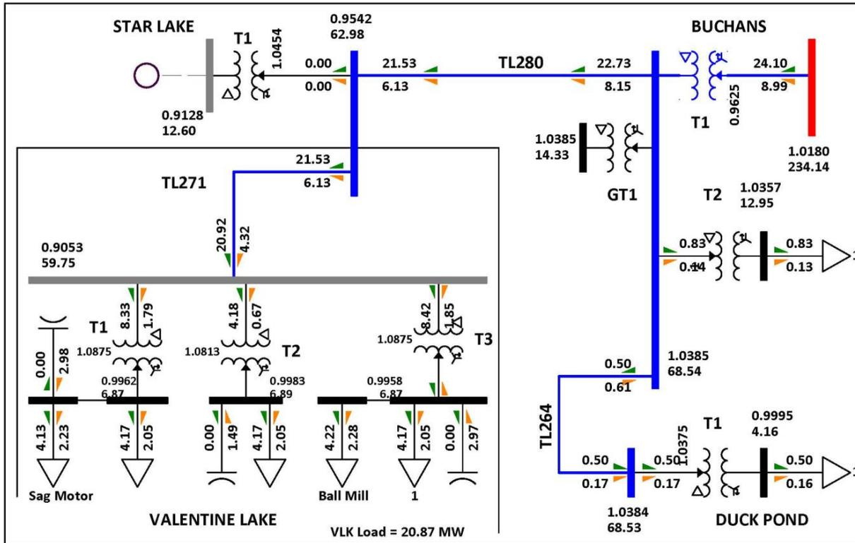
Figure 11: 2024 Light Load Case – SLK out of service
