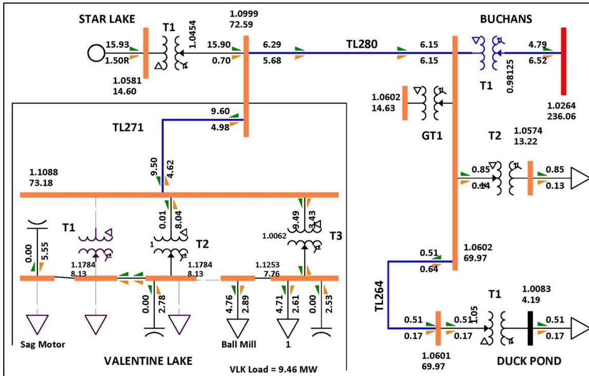
Figure 5: Loss of 11.4 MW of Load at VTN TS
