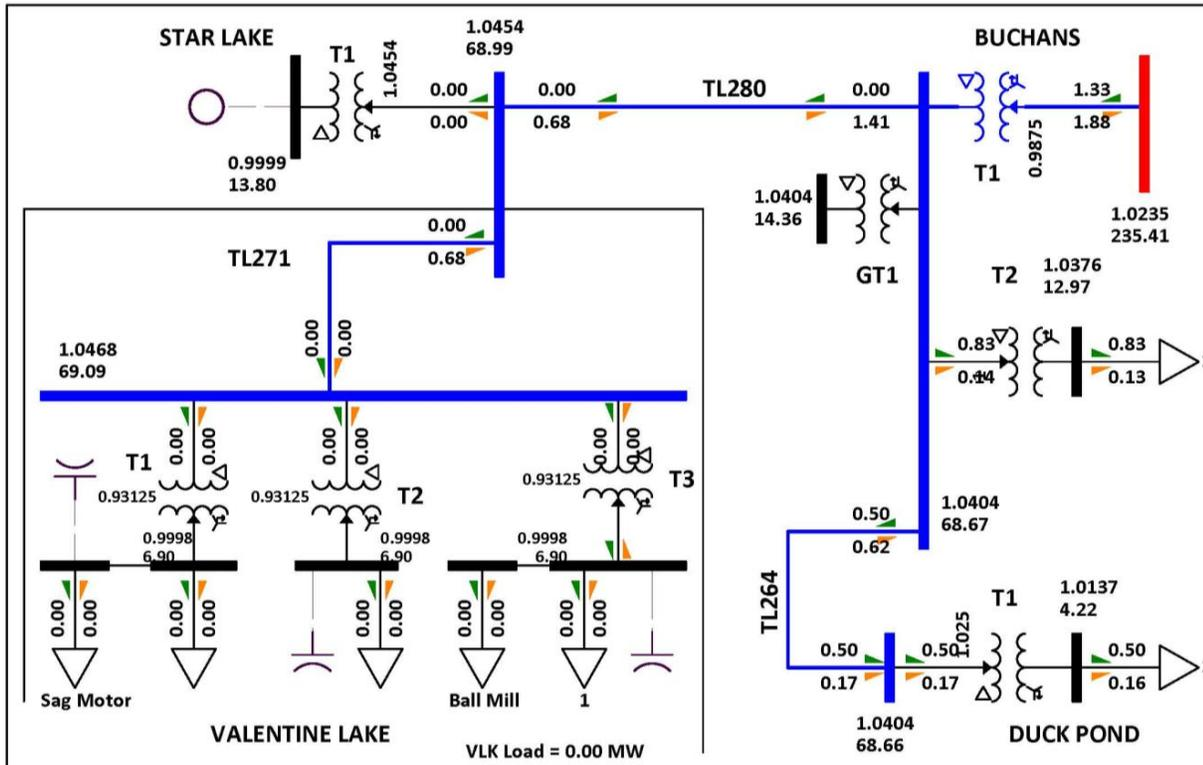
Figure 13: 2024 Light Load Case – N-1 Star Lake Out of Service with No Load at VTN TS
