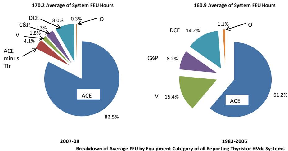
The data for 2007-2008 indicate that the major contributors to the energy unavailability of the converter stations are the converter transformers, followed by the dc smoothing reactors. The provision of a spare unit for these major equipment items greatly improves the availability of the complete converter station, as shown in the following illustrative example.
